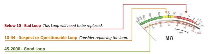
**(Optional) Step 7:** Water down the area of the loop and lead-in and then take another reading. Loops often require water in the groove to facilitate a short to ground. In dry conditions a loop with nicked insulation may still read good. Is your reading significantly lower with water in the groove?
