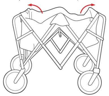
3. Attach the part C bag frame with four-part 1 bolts and four part 2 cap nuts. Secure the part D bag to the frame with the attached Velcro flaps.
