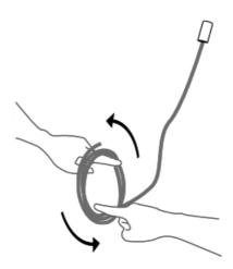
1. Very carefully uncoil the braided coaxial cable in a spool-like manner. Insert your index fingers into opposite sides of the roll then rotate your fingers around each other to unroll the coaxial cable.
