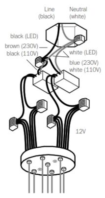
4. Xenon (110V) or LED: connect the black wire to black and white wire to white wire. Xenon (230V): connect black wire to brown wire and white wire to blue wire.
