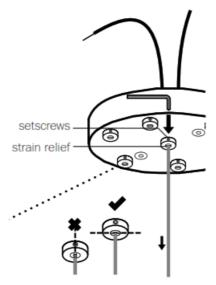
3. Thread the coaxial cables through the canopy, use a 2mm Allen key to loosen the setscrew in the canopy, and gently feed the cable through until you have reached your desired drop length.
