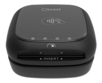
Follow your application instruction to start the transaction process, then swipe, insert or tap card to complete the transaction. If you pay via inserting EMV IC card, please ensure that the EMV chip of the card is facing the right
