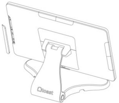
2. Plug in the end of the Micro-USB cable paired with the cover and screws. Then screw in the plate to the terminal.
