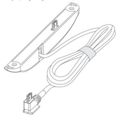
This cable with the plate attached plugs into the side of your terminal and is adhered with screws.
