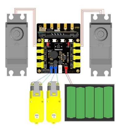
As shown in the figure, PI and P8 are connected to the steering gear (the two power supply short-circuit subshorts are 5V), the L and R motor interfaces are respectively connected to the DC geared motor, and the DC interface is connected to the DC power supply or the battery (the voltage is between 6V and 11.4V). The switch is
