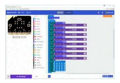
• Expected result: As you push the joystick, the micro: bit display will show an arrow corresponding to the colonted direction
