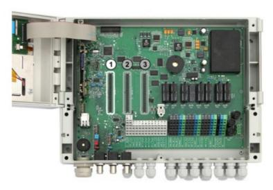
2. Dismantle the cable (or cables) on the required length inside the casing and insert it (them) into the casing through one or more cable glands.
