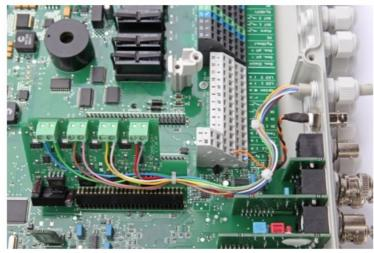
5. Now insert the aluminium rail at its original position. Take care that the PM5-SA4 plug-in module is exactly located in the corresponding slot of the aluminium rail as shown on the second photo below.
