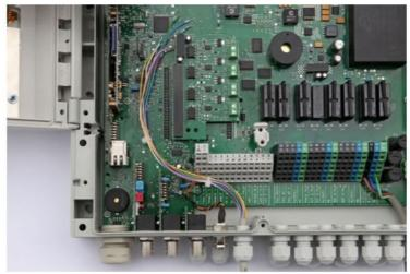
3. Now connect the cable ends to the connection terminals of the PM5-SA4 plug-in module. The digits 1 to 4 indicate the channel numbers which you can later select in the configuration menu.
