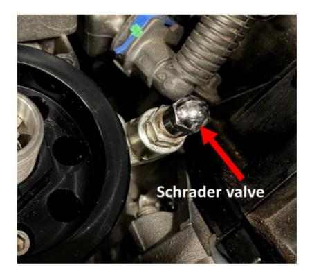
**Helpful Hint:** 90-degree fitting can be installed using a 15/16" 12 point closed end wrench.
