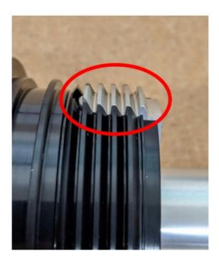
**Step 3:** Lubricate the face seal on the docking collar (body and tip O-rings will be installed later). Install the Adapter until it bottoms out, then back it out less than 180 degrees to expose an NPT port to be utilized for the Schrader valve. Note the orientation (the opposite one will be plugged with the included hex plug) and remove adapter.
