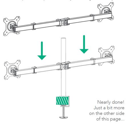
2. Tighten into position at the back, using the supplied 5mm hex key.
