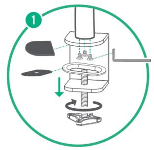
2. Tighten the bracket clamp from beneath by turning the adjuster clockwise and make sure it's tight. Slide the base cover on and clip into place.
