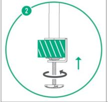
Tighten the bracket clamp from beneath by turning the adjuster clockwise an d make sure it's tight. Slide the base cover on and clip into place.
