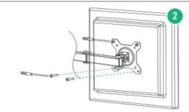
Install the lower two screws. Now you can fasten the upper two
