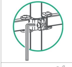
Slide the bracket arms onto the pole. Slide up or down to adjust the height of where your monitors will sit.
