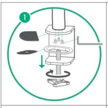
Adhere the bracket clamp cover to the bracket clamp and attach the clamp t o the base with the cap screw. Use the 4mm hex key to tighten.
