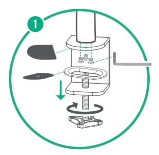
2. Tighten the bracket clamp from beneath by turning the adjuster clockwise and make sure it's tight. Slide the base cover on and clip into place
