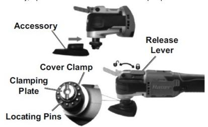
Install the desired accessory by inserting it into the Shaft and placing it onto the Locating Pins.
