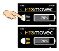
The lights on the bike can be turned on or off using the light icon. The lights can also be accessed via the handlebar unit (see page 5).
