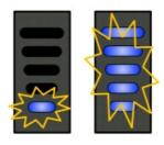
Initially the first LED in the battery indicator (blue) starts to flash as it finds a connection to the battery. When an error is detected all of the LED's will flash. The number of flashes determines the error code.
