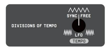
LFO generates cycling triangle and pulse waveforms. Adjust the speed with the LFO knob: to the right for free running, to the left to sync with the tempo.
