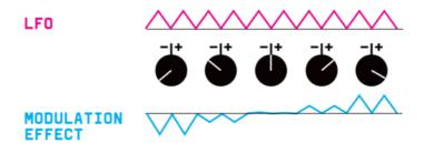
Use MOD to adjust the amount of FEEDBACK modulation. The same goes for TIME and LFO.
