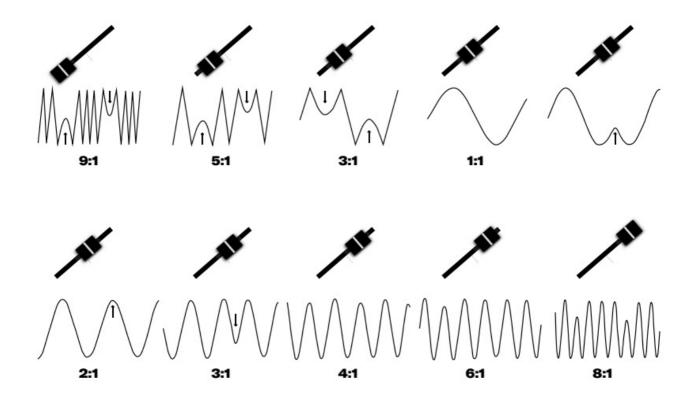
Ranges of both folding algorithms can be extended via CV or by assigning the CTRL knob to FOLD.
