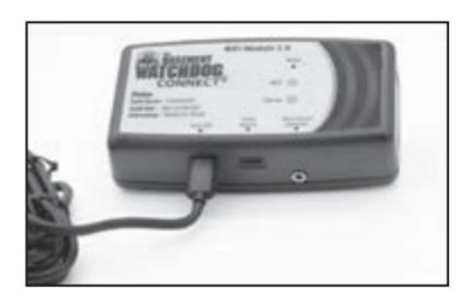
2A-2. Connect the standard USB-A end into the USB port on the backup sump pump controller.
