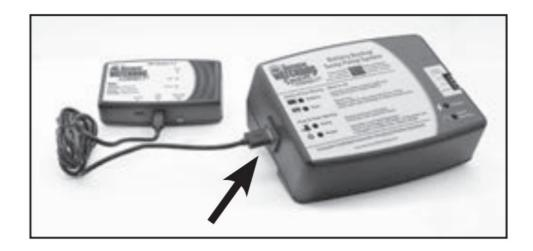
**Note:** When using the Pump System connection, no other cable is necessary; this cable also will power the WiFi Module.
