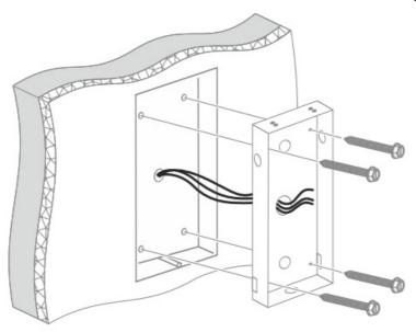
• Cut out a rectangle of 80×40 mm from foamed polyurethane or rubber and make holes opposite the required
