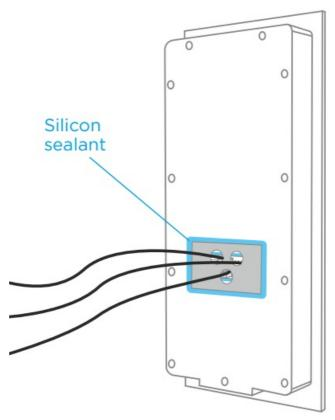
• Apply a 3-4 mm layer of silicone sealant around all wires coming out of the slots in the insulating rectangle. The sealant must be applied to the top of the joint between the wire and the insulating rectangle.
