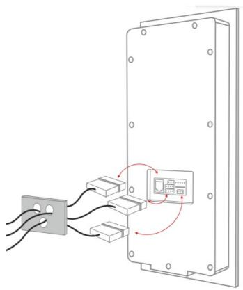
• Apply a 3-4 mm layer of silicone sealant around the niche with the placed insulating rectangle, so that the sealant falls precisely on the joint of the rectangle and the back plastic cover of the panel.
