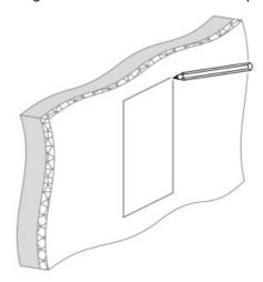
4. Make a niche in the wall by hollowing the wall or any other appropriate way.
