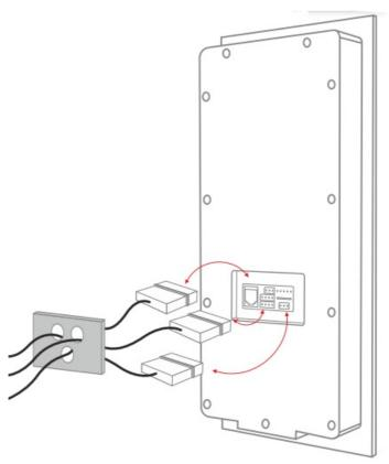
• Apply a thin layer of silicone sealant along the perimeter of the niche with the connectors on the panel rear side and place the protective rectangle in a niche (where all connectors are) on the panel rear side.
