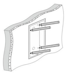
• Remove the bracket and make holes in the outlined places with a perforator.
