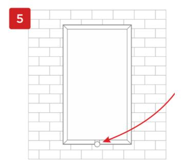
• Place flush mount bracket in the niche and outline places for anchor dowels mount opposite the holes in the bracket.
