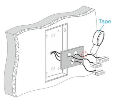
• Join all the resulting connectors at the ends of the wires to their corresponding response parts on the panel rear side.
