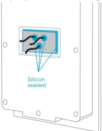
• Put all connected to the panel wires on the bottom of the flush mount bracket. All the protruding from the wall and connected to the panel wires must be carefully bent in a semicircle in so that the upper part of the wiring bundle is higher than the hole for inserting cables from the wall into the inside of the bracket.
