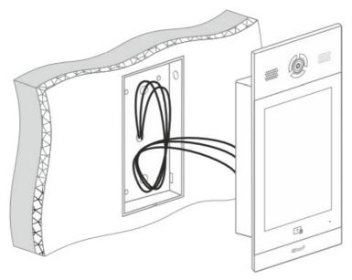
• Install the entrance panel inside the flush mount bracket.
