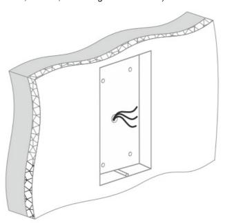
• Place the flush mount bracket in the hollowed-out niche and fasten it with screws through the mounting holes.
