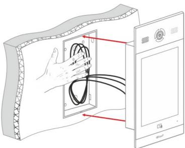
• Fasten the entrance panel to the bracket with the fastening bolts from the kit.
