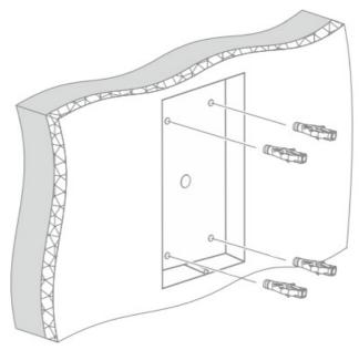
• Wire all the necessary cables for panel connection and switching (for Ethernet, an exit button, a lock, panel power, a door sensor, a fire alarm, RS485, and Wiegand interfaces) into the niche.
