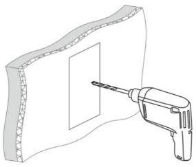
**Attention:** the hole at the bottom is designed to drain the water. Do not intentionally close it. Also it is necessary to make a drain for water at the bottom of the niche which will serve to divert water out.
