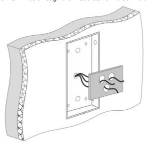
• Switch and connect the protruding from the wall and passing through the insulating rectangle wires to the necessary connection cords from the panel kit.
