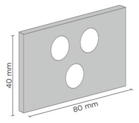
• Pass all the protruding from the wall wires through the made earlier holes in the insulating rectangle.
