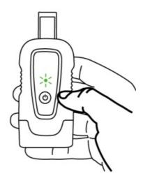
**Note,** to conserve battery, the Tool will automatically power off if the tread depth measurement reading does not change for a period of 30 seconds. In this case, press the power button to turn the Tool on again
