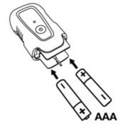
4. Press firmly on either side of the end cap, align the casing & push inwards until it clicks into place
