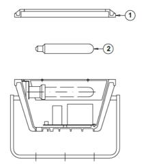
By choosing the desired angle bracket acting on the side screws, then tighten fully. Fix the floodlight by adequate stainless steel screws, using the proper holes on the fitting bracket.
