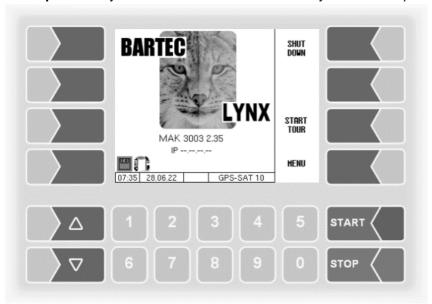
The system offers so called **hidden functions.** To display the hidden panel press any of the four left soft keys. The EVENTS and LAST TOUR functions become visible. Press the soft key labeled with the desired function within three seconds to enter it. If you do not press any soft key the hidden panel will disappear automatically.
