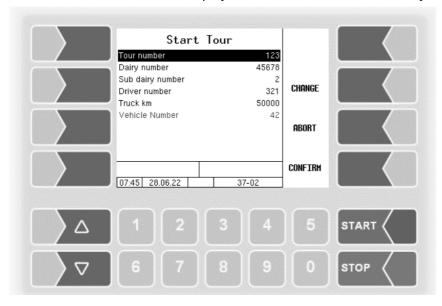
3. The Tour Details screen will appear. This screen has hidden functions on both sides. Activate the hidden MENU function by pressing any right soft key → the MENU function becomes visible and has to be pressed within 3 seconds to activate.
