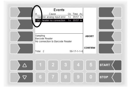
To leave the EVENTS screen you have to activate the hidden panel by pressing any of the left soft key first. Press EXIT within 3 seconds to return to the home screen.
