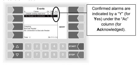
The "BC-Reader no connection" alarm is still active, but has been marked as acknowledged by the user. Please observe that the CONFIRM soft key has vanished once the alarm has been confirmed. If the problem that caused the alarm is fixed, the acknowledged alarm will be automatically removed from the EVENTS list.
