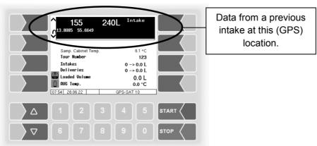
4. The system waits for milk to be sucked in. You can abort the intake by pressing ABORT as long as no milk has been detected – once milk has been detected, the ABORT soft key will disappear.
