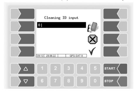
5. The System is now ready to start the CIP process. The valves will start to alternate after flow is detected.
