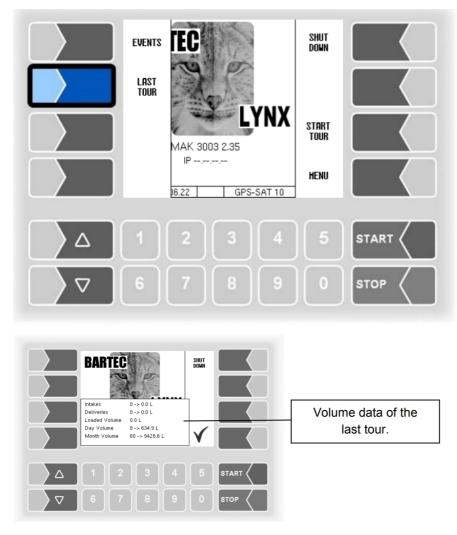
4. To turn off the system, press SHUT DOWN.
