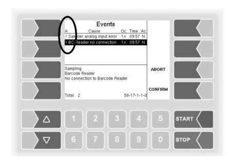
Here you can see the EVENTS screen with two active alarms. Active alarms are indicated by an exclamation mark under the "A" column.
