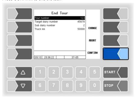
3. You will return to the home screen. To view data of your last tour, activate the hidden LAST TOUR function by pressing any left soft key the LAST TOUR function becomes visible and has to be pressed within 3 seconds to activate.
