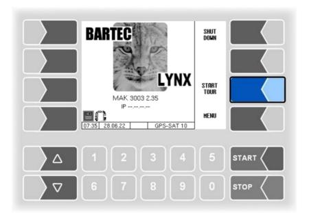
2. The Start Tour screen will appear. Before you can start a tour it is necessary to set the entries displayed on the screen. You can navigate through the entries with the selection keys at the bottom left of the operating unit. To set an entry press CHANGE (or any numeric key). Press CONFIRM to start the tour.
