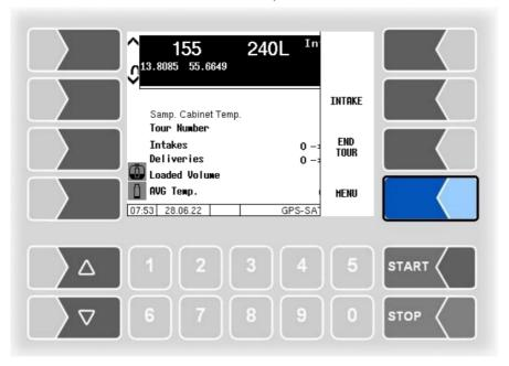
2. The **Tour Menu** screen will appear. Select **Emptying System** with the selection keys and press ENTER. The pump will suck air to press the remaining milk from the system into the trailer.
