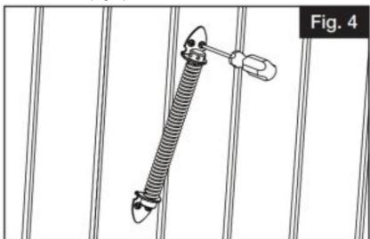
c. To increase tension, close the gate and use provided adjustment rod to turn the tensioned barrel a maximum of 3 increments. Holding the rod in place, insert the tension pin in the open slot closest to the post on the side opposite of the gate (Fig. 5).
