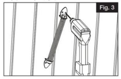
b. Fasten spring with provided screws (Fig. 4).
