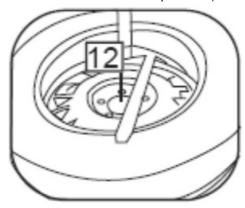
Final inspection: Visually inspect the rim, valve stem, and electronic module to ensure no damage has occurred.
