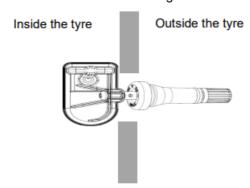
Place the Self-lock Screw<sup>①</sup> on the valve stem, and tighten with 5 Nm (44-inch pounds) torque.
