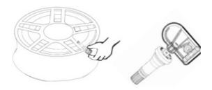
Remove the Self-lock Screw①, and insert the valve stem through the rim hole from inside.
