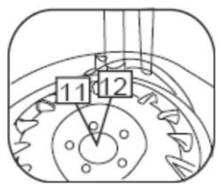
Use the same procedure to dismount the lower tire bead. (If the mounting head of the tyre changer is at the noon position, then the valves stem should also be at the 12 o'clock position.)
