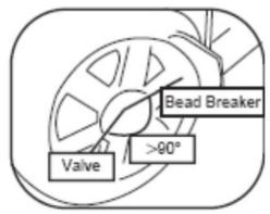
Firmly fix the wheel on the turntable clamps. (If the mounting head of the tyre changer is positioned at noon, then the valves stem should be at the 11 o'clock position.) Apply lubricant to both tyre bead and rim, and then remove the upper tyre bead.
