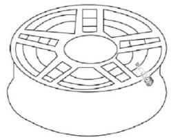
Lock the rim on the tire changer. (If the mounting head of the tire changer is positioned at noon, then the valve should be at the 7 o'clock position.) Apply lubricant on both the tire bead and rim. Mount the lower tire bead on the rim. Ensure that the tire bead does not touch the electronic module during mounting.
