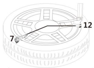
Mount the upper tyre bead the same way. (If the mounting head of the tire changer is positioned at midnight, then the valve should be at the 5 o'clock position.) Inflate the tire to nominal pressure.
