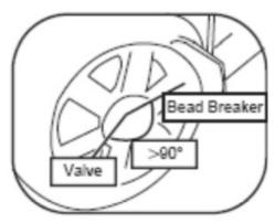
2. Firmly fix the wheel on the turntable clamps. (If the mounting head of the tyre changer is positioned at 12 o'clock, then the valves stem should be at the 11 o'clock position.) Apply lubricant to both tyre bead and rim, and then remove the upper tyre bead.
