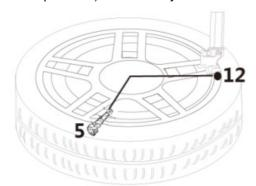
7. Apply soapsuds on the valve tip. If no leakage is found, put on the valve capo6. If unsuccessful, try again.
