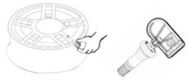
3. Remove the Self-lock Screw①, insert the valve stem through the rim hole from inside.
