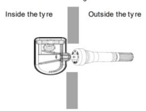
4. Place the Self-lock Screw①on the valve stem, and tighten with 5 Nm (44 inch-pounds) torque.
