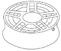
5. Lock the rim on the tire changer. (If the mounting head of the tire changer is positioned at 12 o'clock, then the valve should be at the 7 o'clock position.) Apply lubricant on both the tire bead and rim. Mount the lower tire bead on the rim. Ensure that the tire bead does not touch the electronic module during mounting.
