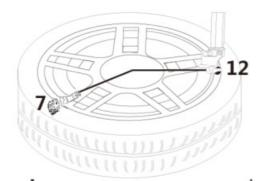
6. Mount the upper tire bead the same way. (If the mounting head of the tire changer is positioned at 12 o'clock, then the valve should be at the 5 o'clock position.) Inflate the tyre to nominal pressure.
