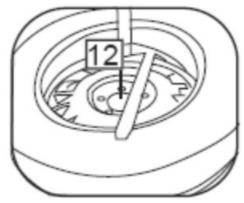
4. Final inspection: Visually inspect the rim, valve stem, and electronic module to ensure no damage has occurred.
