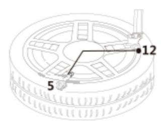
1.7 Apply soapsuds on the valve tip. If no leakage is found, put on the valve capo6. If unsuccessful, try again.
