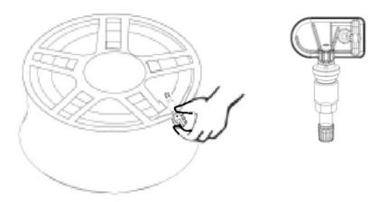
1.3 Take off the nut , insert the valve stem through the rim hole from inside.
