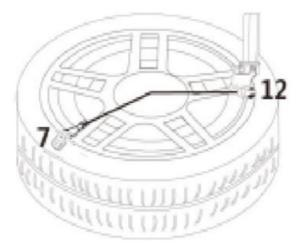
1.6 Mount the upper tyre bead the same way. (If the mounting head of the tyre changer is positioned at 12 o'clock, then the valve should be at the 5 o'clock position.) Inflate the tyre to nominal pressure.
