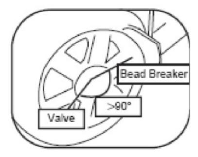
2. Firmly fix the wheel on the turntable clamps. (If the mounting head of the tyre changer is positioned at 12 o'clock, then the valves stem should be at the 11 o'clock position.) Apply lubricant to both tyre bead and rim, and then remove the upper tyre bead.
