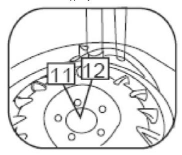
3. Use the same procedure to dismount the lower tyre bead. (If the mounting head of the tyre changer is at the 12 o'clock position, then the valves stem should also be at the 12 o'clock position.)
