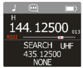
3. You can press the key to save the Search frequency and CTCSS or DCS to the channel.
