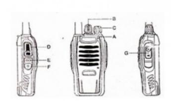
A LED Indicator Lights red during transmit, green when receiving a signal
