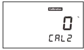
• Place the dissolved oxygen electrode into the zero oxygen solution. for about 10 minutes.
