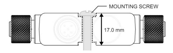
**CAUTION:** Do not overtighten the R95C's mounting screw during installation. Overtightening can affect the performance of the R95C.
