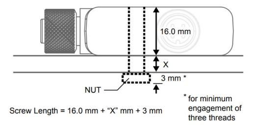
CAUTION: Do not overtighten the R90C 4-Port Hub's mounting screw during installation. Overtightening can affect the performance of the R90C 4-Port Hub.
