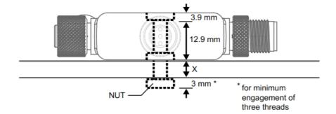
Screw Length (with screw head fitting in counterbore) = 12.9 mm + "X" mm + 3 mm
