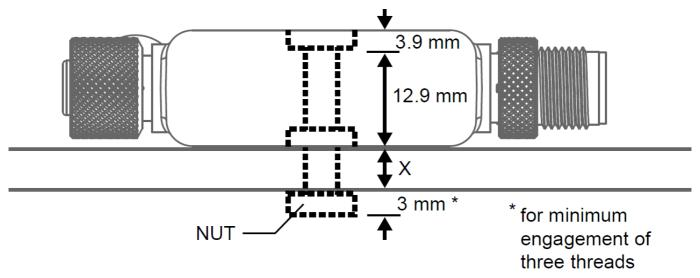
Screw Length (with screw head fitting in counterbore) = 12.9 mm + "X" mm + 3 mm
