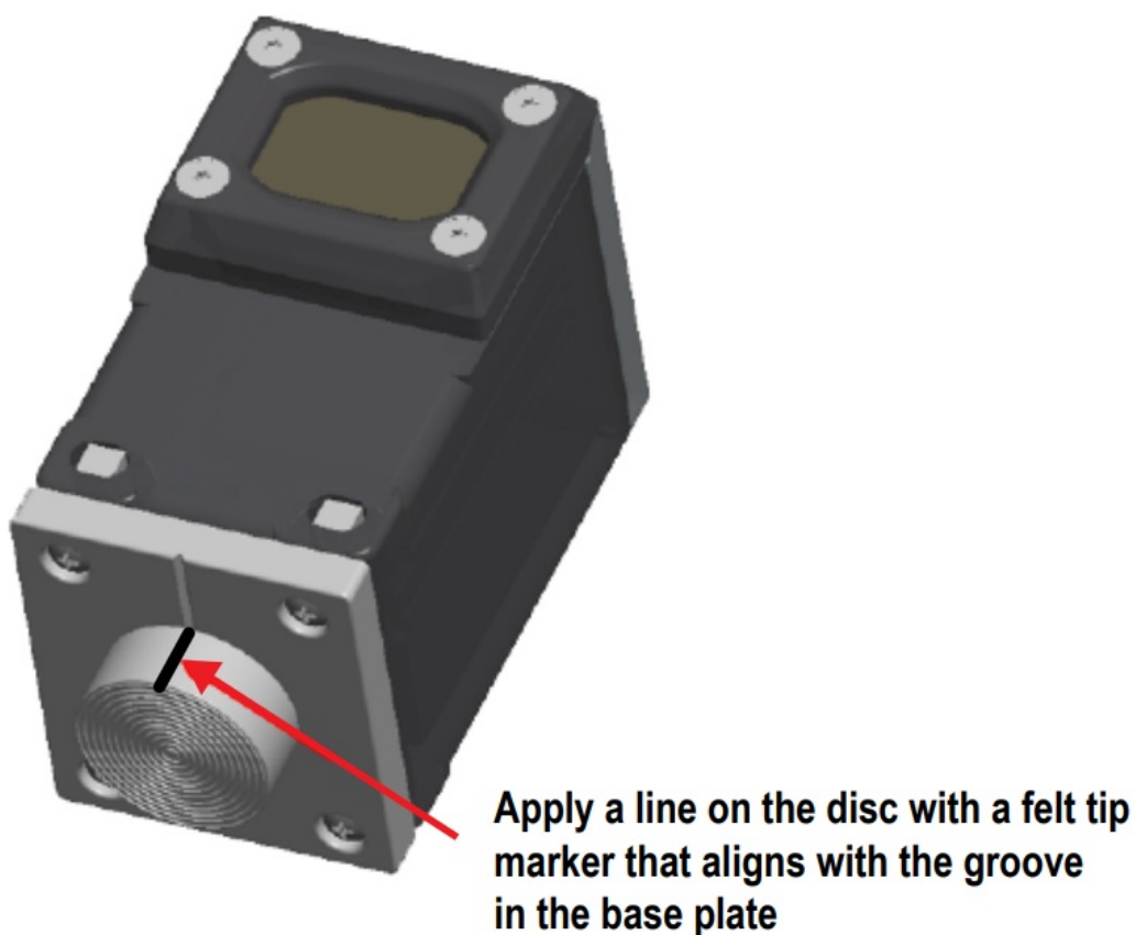
Figure 10. Place a mark on the disc
