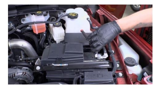
If you rush this step and unplug the MAP sensor, it can flag a Check Engine Light in the ECM on startup.
