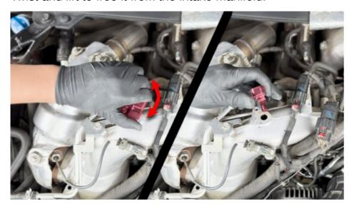
Due to the sensitivity of the sensor, GM advises not to use any chemical cleaners, including water, and not to use compressed air to remove contaminates. Proceed with cleaning the sensor at your own risk.
