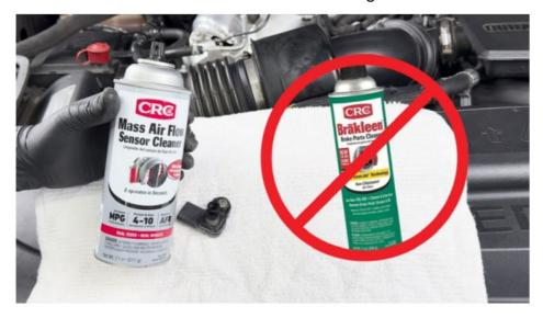
While GM does not recommend cleaning, we have seen favorable results using Mass Air Flow (MAF) Sensor Cleaner, available at most auto parts stores.
