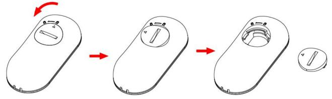
2. Put a 3V button battery of model "CR2032" or "CR2025" into the battery box as shown in the figure, the protruding metal tips clamp one side of the battery and the finger presses the battery into the battery box. Please note that the battery "+" should face us; Place the cover back and lock it by rotating 90° clockwise.
