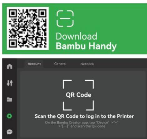
3. Use Bambu Handy to scan the QR code on the screen, and bind your printer with your Bambu Lab account.
