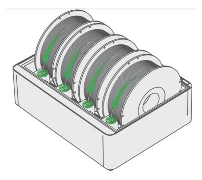
Place at least one spool of Bambu Filament into the AMS. Turn on the power to start the printer and the AMS. Insert the filament into the filament inlet. The filament will be automatically pre-loaded when detected.
