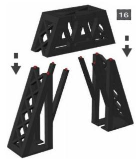
• Apply glue on the "red" surface to assemble the mating part.
