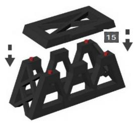
• Apply glue on the "red" surface to assemble the mating part.
