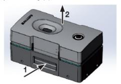
2. Remove battery (1) and insert new battery with correct polarity (2). The poles are marked with "+" and "-".
