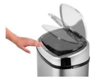
To open the bin. hold your hand 5-20cm above the lid and it will automatically open within half a second. Once your hand is removed from the sensor area it will automatically close within 5-6 seconds. Keeping your hand within the sensor area will keep the lid open. Alternatively you can press the 'open' Button to lift the lid bur it will not close For 90 seconds unless you press 'close
