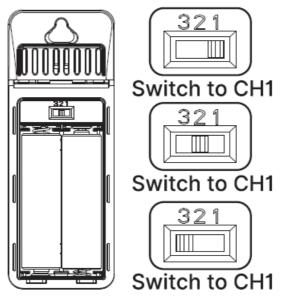
2. Load the 2xAA batteries in 3 minutes to ensure RF signal received in time.
