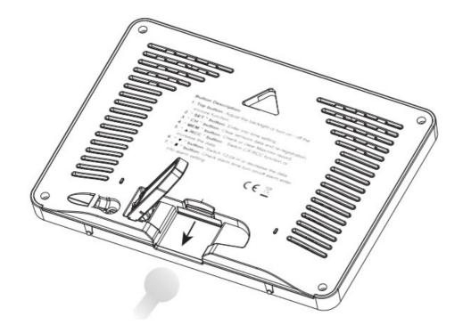
Step 3, Remove the built-in cell battery insulation strip.
