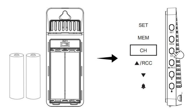
If not powered on within 3 minutes from the main unit powered on. Press and hold the "CH" button for 3 seconds to search the RF signal again.
