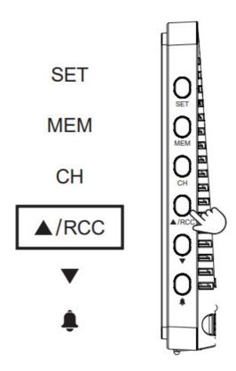
Press & hold the ▲/RCC button will allow exiting the Atomic mode to continue manual setup.
