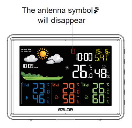
Press and hold "▲/RCC " button for 3 seconds to search RCC radio signal again
