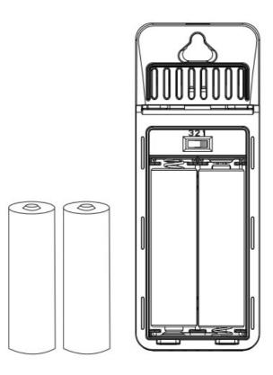
Step 2, Load the 2xAA batteries to each sensor within 3 minutes to ensure the RF signal is received in time.
