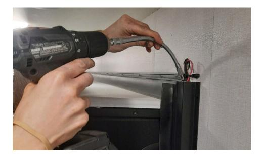
Use the flex shaft and #3 square bit provided. Locate each motor at the top of the mechanism. Insert the drive bit into the end of the motor and activate with a cordless drill (DO NOT USE AN IMPACT DRIVER). Alternate between motors so that the room does not become wedged in the opening or encounter cabinets or other fixtures in the RV.
