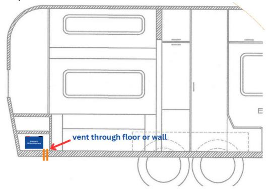
**Example 2:** Installed outside the structure in an enclosure, i.e. under the floor, on the drawbar **Requirements for install:**
