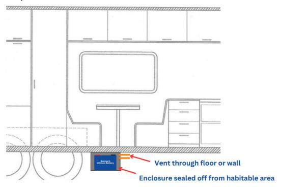
**Example 3**: Installed in a space that is not part of the habitable area and only accessible internally, eg Under bed, Under seat, Inside cupboard.
