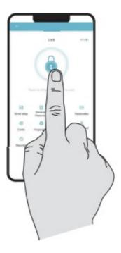
• To unlock the lock, tap this icon once. To lock the lock, press and hold on this icon.
