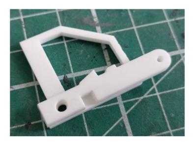
**Step Eight.** Glue the two assemblies together using 12 positioned in the slots on 10. Check that the front pivot aligns with the pivots on the main bed, adjust if necessary.
