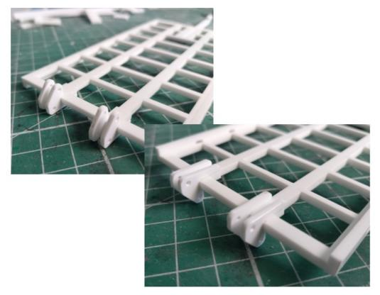
**Step Seven.** The rear chassis starts by gluing 10 on top of 5. Ensure the axle hole lines up and the two parts are parallel. Repeat for the other side making sure to glue **the opposite way round!**
