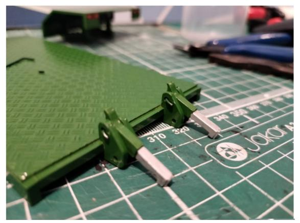
**Step Eighteen.** Slot the longer pin through the **lower** pivots and the rear frame to connect the two. Again lock in place by gently bending the end over.
