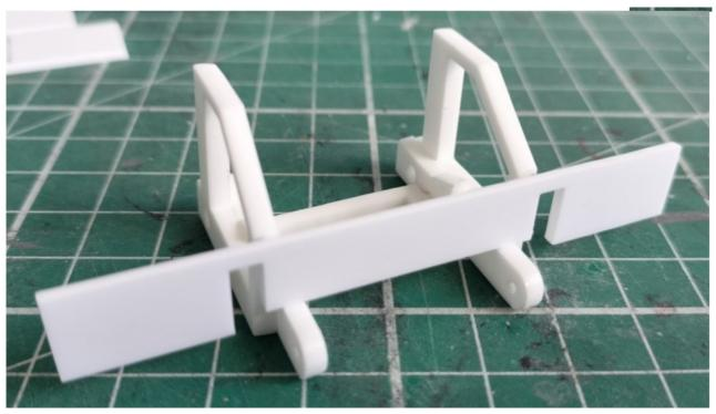
**Step Ten.** Add the second panel 7 on the angle and finish with the top panel 8. **Note:** You may wish to glue the two chocks onto panel 7 now, or you can paint them separately and glue on later.
