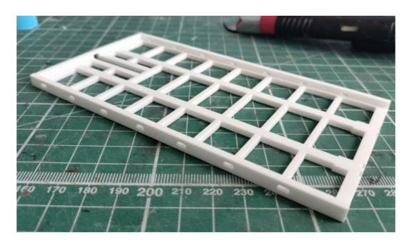
**Step Four.** Assemble the tow beam. Glue the two 2's back to back and then add the tow eye 14 to the top of the sloped end as pictured.
