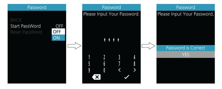
After entering your desired 4-digit code, you must re-enter the 4-digits you chose, to ensure the code is correct. Then the interface exit back automatically to original interface within two seconds.
