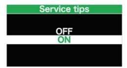
**Note:** The default setting is OFF. If the ODO is more than 5000 km, the "Service" indication and mileage indication will flash for 4S.
