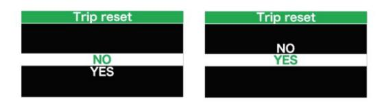
Note: The riding time(TIME), average speed (AVG) and maximum speed (MAXS) will be reset simultaneously
