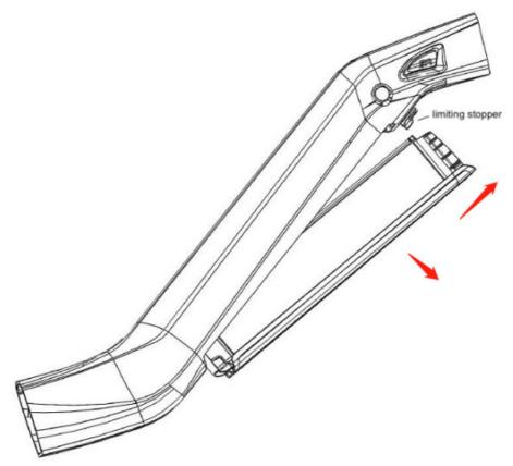
2. Push the top part of the battery into the frame, until you hear the battery lock into position, and turn the limiting stopper to keep the battery from dropping.
