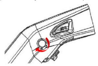
2. Push the limiting stopper to release the second locking mechanism and take off the battery.
